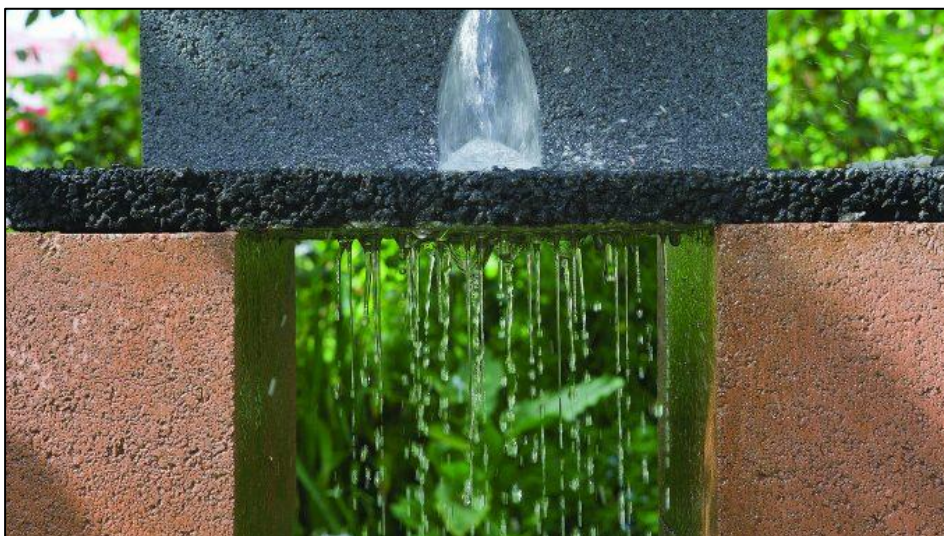
Figur 9. Infiltration genom permeabel asfalt (Magazine.ogind.com, 2018).
